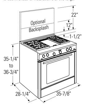
Clearances between range and side wall or combustible material must be at least 12" on each side.
